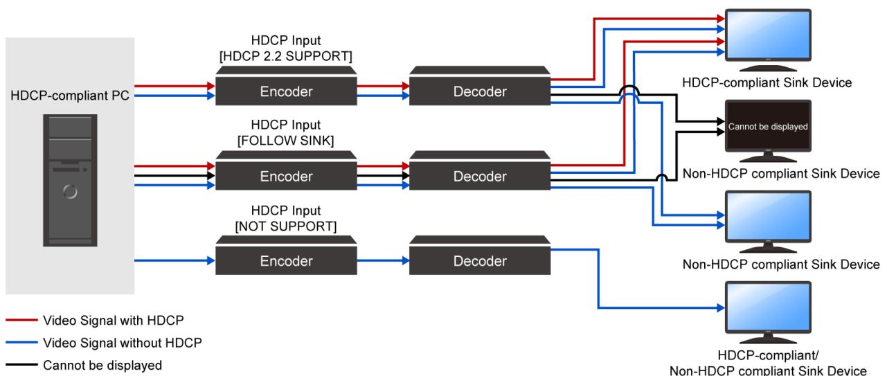
To enable this setting, set “**Disabling HDCP or EDID settings (P.12)**” of DIP switch No.3 to [OFF].
