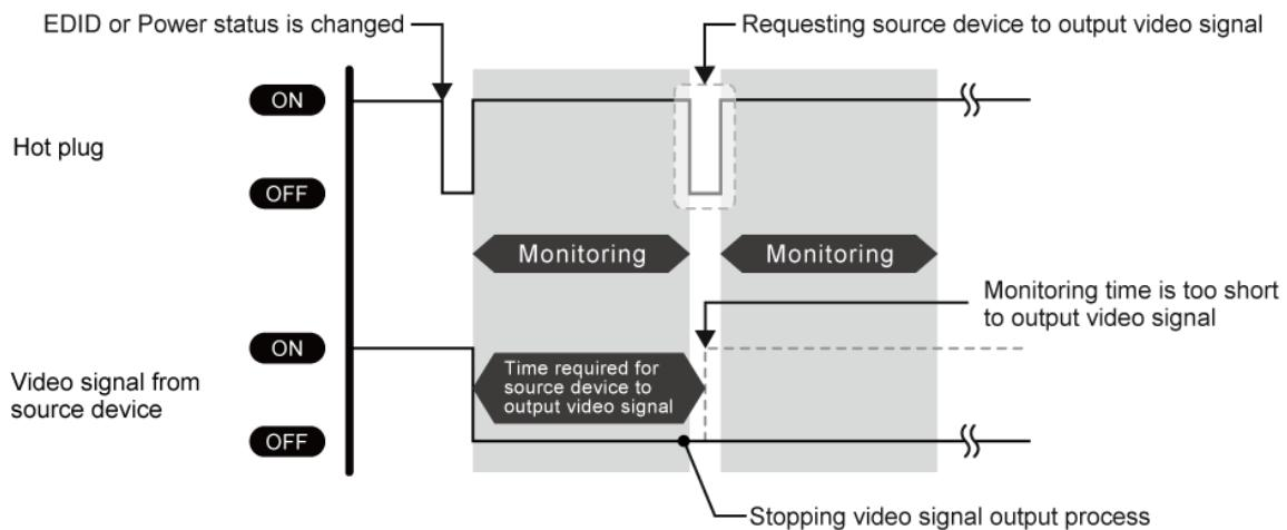
If the interval is shorter than the time for source device output video signal, the source device repeats the video output process and does not output video signal. This problem can be solved by setting longer monitoring time.
