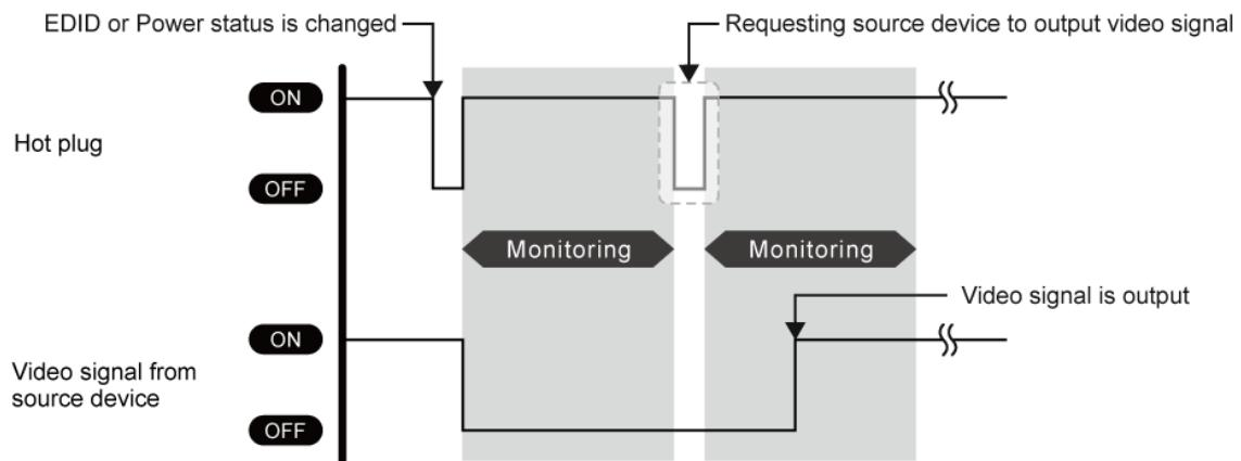
■ Example: The specified monitoring time is too short. → Set the longer monitoring time.
