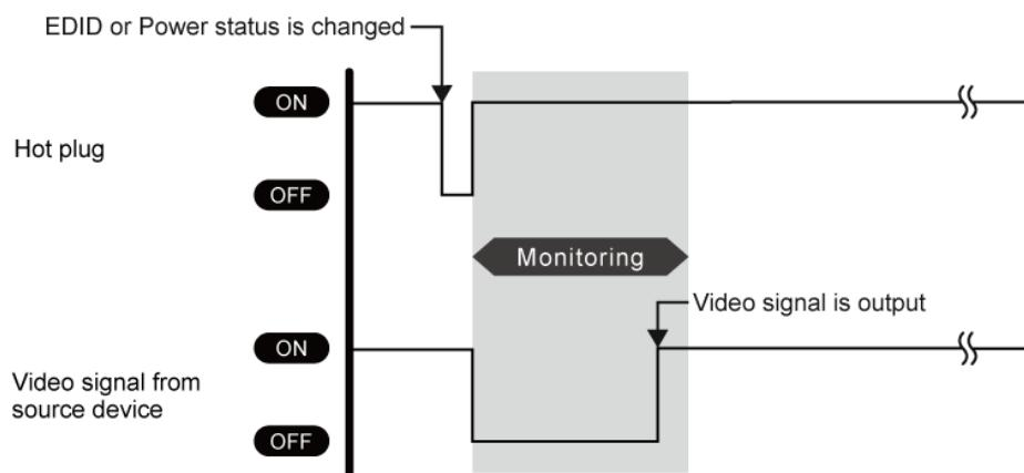
■ Example: The source device stops outputting video signals → Hot plug request is needed.
