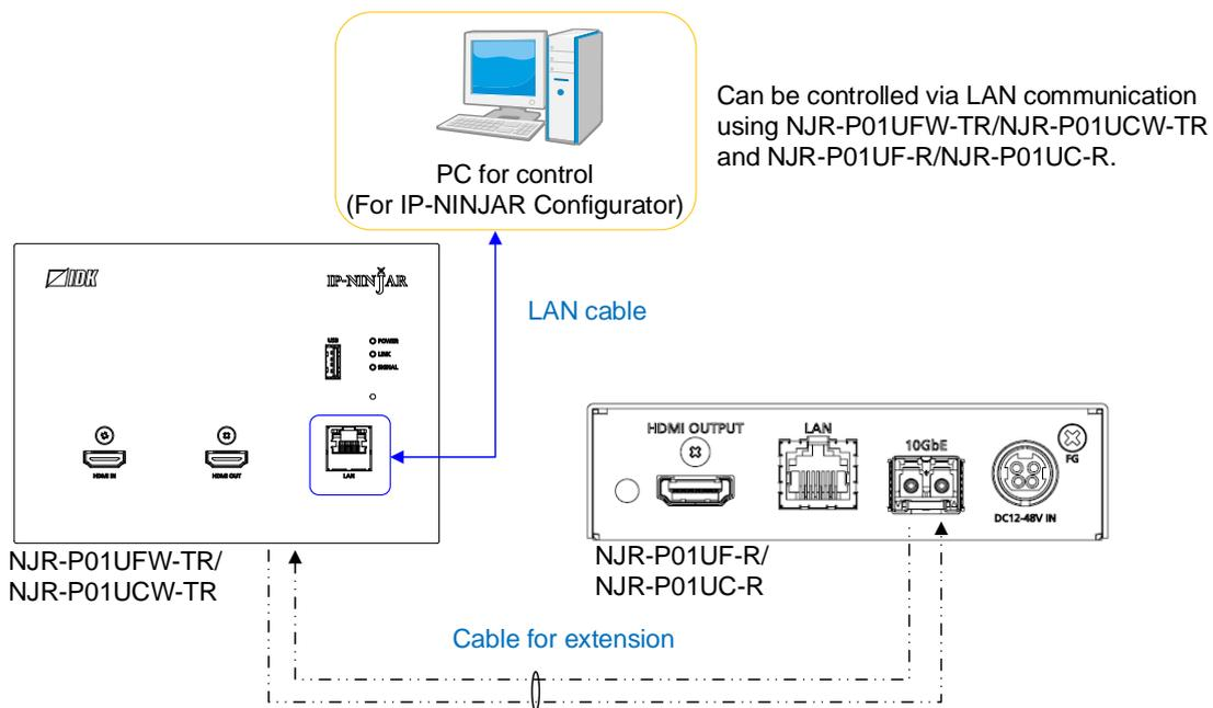
[Fig. 3.3] Connecting to LAN cable
