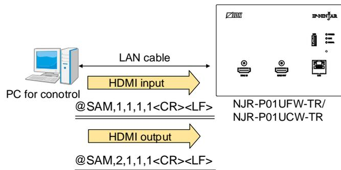
[Fig. 4.2] Command input from IP-NINJAR Configurator
