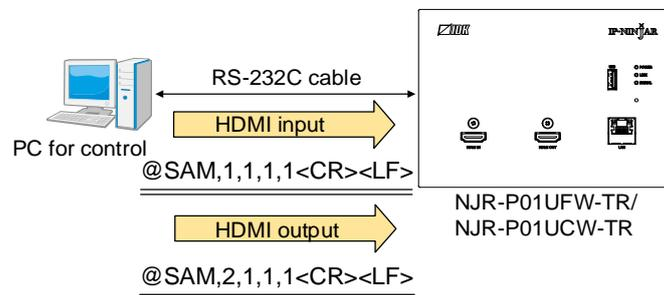
[Fig. 4.1] Command input from RS-232C
