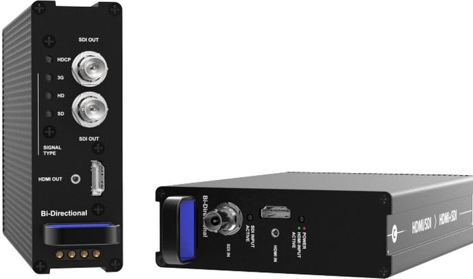
The SDI/HDMI Bidirectional Reversible Module fits in the 8-Bay Reversible Rackmount Converter system.
